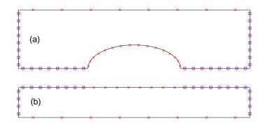
FIG. 3.2. The boundary integral method is applied to the domain  $D_1 = \Omega_2^m$  (upper panel) and the domain  $D_2 = \Omega_3$  (lower panel) separately. The electrostatic potential  $\Phi$  and its directional derivative  $\Psi$  are evaluated at the discrete points indicated by " $\circ$ " and " $\times$ " respectively along the boundaries.
