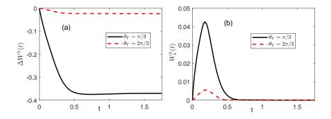
FIG. 4.6. The energy loss  $\Delta W(t) = W(t) - W(0)$  (left panel) and the kinetic energy  $W_k(t) = \frac{1}{2} \int_{\Omega} \rho |\mathbf{u}|^2 d\mathcal{L}^2$  (right panel) as functions of time. Here the discrete energy W(t) is computed using the dimensionless from of (A.2).
