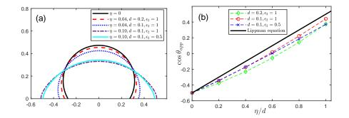
FIG. 4.3. Left panel: Equilibrium profiles of the interface. Right panel: The value of  $\cos \theta_{app}$  versus  $\eta/d$  (discrete points with dash lines) and the prediction of Lippmann equation (straight line).
