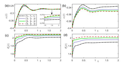
FIG. 4.2. The evolution of the (left) contact point (upper panels) and the contact angle (lower panels) computed using different mesh sizes and time steps. In the coarse mesh, the mesh size is  $h = h_0 = 1/32$  for the interface and  $h_{\Omega} = h_1 = 1/8$  in the bulk, and the time step is  $\tau_0 = 0.01$ . Left panels:  $\eta = 0$ ; Right panels:  $\eta = 0.1$ .
