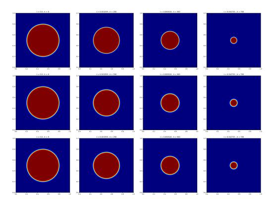
FIGURE 8. Comparison of the numerical semigroups  $\mathcal{S}^{AC}_{\delta_t,\varepsilon,1}$ ,  $\mathcal{S}^{NN}_{\theta,1}$  and  $\mathcal{S}^{NN}_{\theta,2}$  for the approximation of the mean curvature flow of a circle; each row corresponds to the evolution obtained at different times using, respectively, the numerical semigroup  $\mathcal{S}^{AC}_{\delta_t,\varepsilon,1}$  and the networks  $\mathcal{S}^{NN}_{\theta,1}$  and  $\mathcal{S}^{NN}_{\theta,2}$ .
