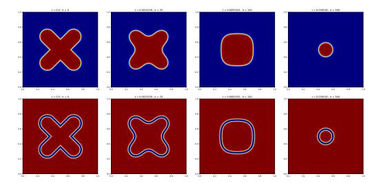
FIGURE 16. Approximation of the mean curvature flow of a non convex initial set: numerical comparison of the classical discretisation of the Allen-Cahn equation  $\mathcal{S}^{\text{AC}}_{\delta_t=\varepsilon^2,\varepsilon,1}$  (first line) with the network  $\mathcal{S}^{\text{NN}}_{\theta,2}$  trained on the non oriented phase field  $q'(\text{dist}(x,\Gamma)/\varepsilon)$  (second line). In each line, we plot the solution  $u^n$  at different times  $t_n$ .
