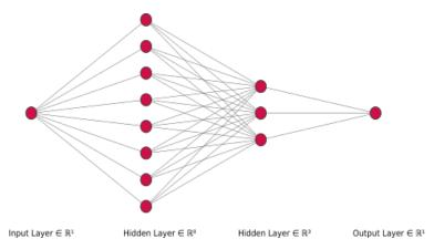
FIGURE 6. Reaction network based on a 1D multilayer perceptron using two hidden layers with respectively 8 and 3 neurons.
