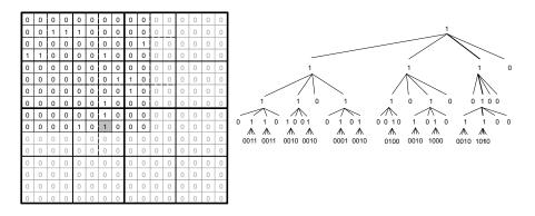
Figure 1: A set of points, indicated by 1s, on a  $16 \times 16$  grid (left); the quadtree for those points (right). The heavy lines in the quadtree indicate the path to the leaf corresponding to the shaded point on the grid.
