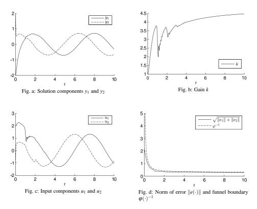
Fig. 8.2: Simulation of the funnel controller (7.2) with funnel boundary specified in (8.2) and reference signal  $y_{\text{ref}} = (\sin, \cos)^{\top}$  applied to system [E, A, B, C] with initial data (8.1).
