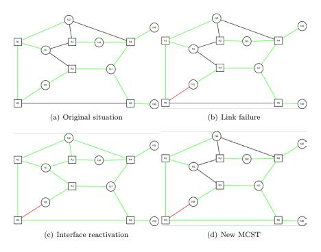
Fig. 16: GOSPF dealing with a link failure through a RESET operation
