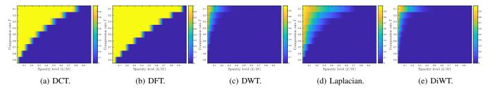
Fig. 4: Phase transition analysis of CS matrix  $A = \Phi \Psi$  for different bases, where  $\Phi$  is the proposed measurement matrix and  $\Psi$  is the basis matrix. The color bar indicates successful recovery probability  $P_s$ . CS matrix A with DCT and DFT basis yields promising recovery region.
