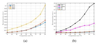
Fig. 8: Average reconstruction error against different compression rates. Here, 1024 temperature data points are considered. Figures (a) and (b) depicts recovery of grid-wise and Randomly deployed nodes measured data respectively. DFT basis provides low recovery error compared to all bases in both grid and random deployment scenario.
