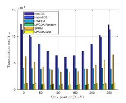
Fig. 13: Comparison of the transmission cost required for data aggregation from 625 nodes deployed in an area of  $256m \times 256m$  using the proposed LWCDA and SPRM, Hybrid CS, CWCDA and Non-CS methods against the sink location. The sink node location (X, Y) varies according to the line X = Y where  $X, Y \in [0, 256]$ . Transmission cost of the proposed LWCDA method is robust and lower compared to all baseline approaches for all considered sink locations.
