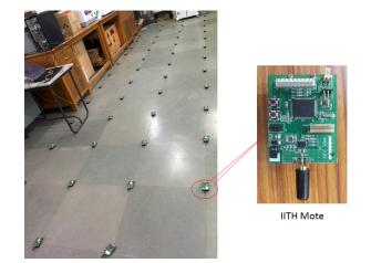
Fig. 14: Experimental setup with N = 50 nodes deployed in an area of  $321.44 \ ft^2$ .
