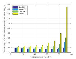
Fig. 10: Comparison of the percentage of disbursed transmission cost of the proposed LWCDA with respect to SPRM, Hybrid CS, CWCDA and Non-CS methods against the compression rate  $\Gamma$ . Here, data aggregation is considered from 625 nodes deployed in an area  $256m \times 256m$ . Percentage of disbursed transmission cost of the LWCDA with respect to SPRM, Hybrid CS, CWCDA and Non-CS methods is low for almost all compression rates ( $\Gamma < 80\%$ ).
