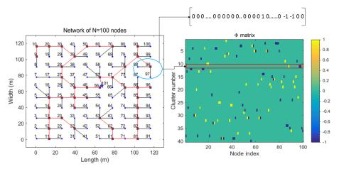
Fig. 1: The procedure of measurement matrix designing from a network with N = 100 nodes and M = 40. The sink S = 101 is represented by a star, square boxes represent the CHs and remaining nodes are leaf nodes.
