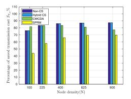
Fig. 12: Comparison of the percentage of saved transmission cost of the proposed LWCDA with respect to SPRM, Hybrid CS, CWCDA and Non-CS methods against node density at  $\Gamma = 50\%$ . Here, an area of  $256m \times 256m$  is considered for the network deployment and number of nodes (N) deployed are varied. The proposed LWCDA method offers savings in the transmission cost consistently with respect to the baseline approaches for all the considered node densities.
