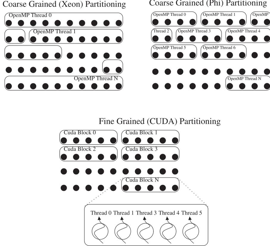
Fig. 4. Fine-grained and coarse-grained distributions of the lattice notes.
