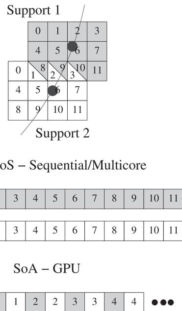
Fig. 7. Different data layouts used to store the information about the coordinates, velocities and forces of the *Lagrangian* points and their supports. On multi-core processors we use an AoS data structure (top) whereas on GPUs (bottom) we use a SoA data structure.
