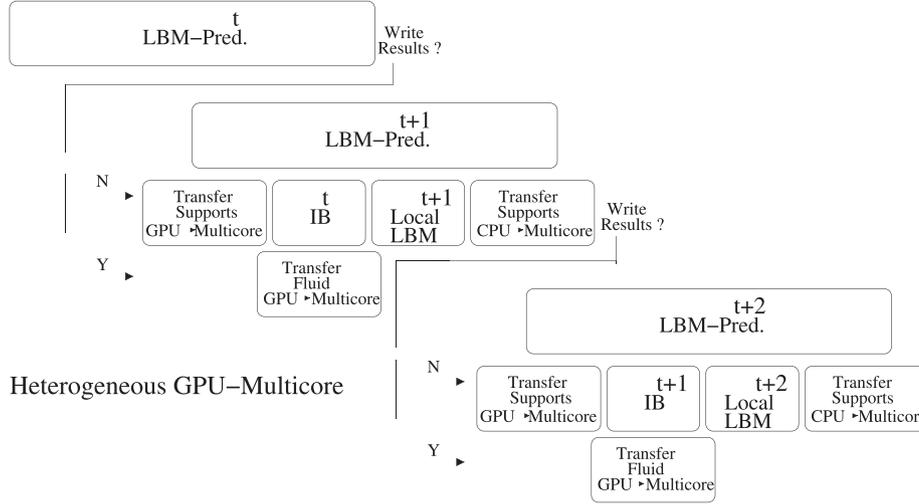
**Fig. 9.** Hybrid multicore-GPU implementation. The LBM update is performed on the GPU, whereas the IB correction and an additional step to update the supports of the Lagrangian points are performed on the multi-core processor.
