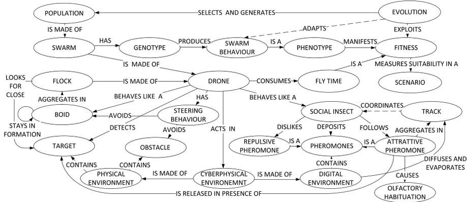
Figure 6: Ontology of the FSE swarming algorithm.
