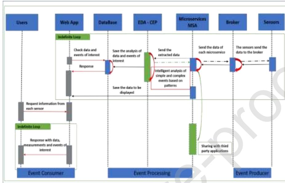
Figure 3.4. Sequence diagram of event flow in IA-CPS specification and data query from client-side.
