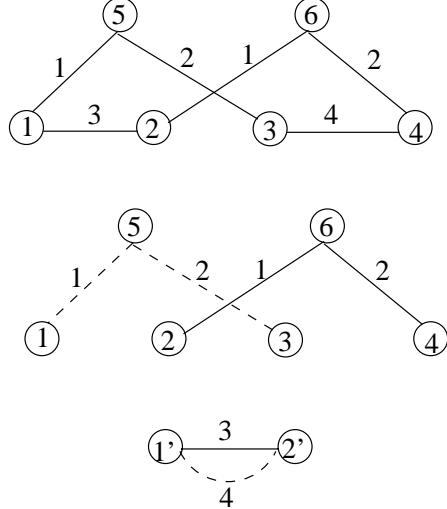
Figure 2: Example of the race condition between two processors when Boruvka’s algorithm is used to solve the MST problem.
