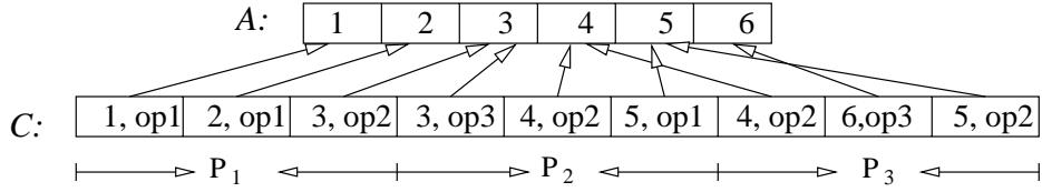
Figure 1: Conflicts when partitioning work among the processors. Here for simplicity we assume every condition in  $C$  is true and they are not shown.
