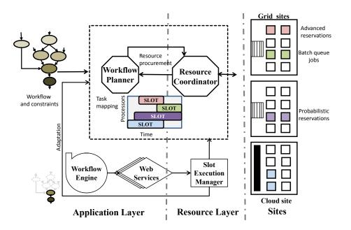
Figure 1: WORDS Architecture introduces a clean separation between resource level and application-level functionalities through a resource abstraction(slot). The workflow planner interacts with the resource coordinator to facilitate resource procurement.
