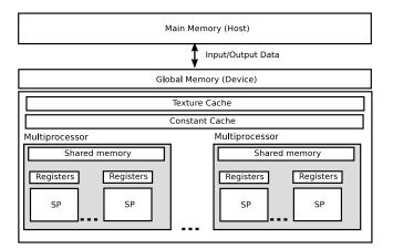
Figure 1: General Purpose GPU Architecture. (SP: Streaming Multi-Processor)
