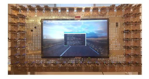
Figure 5: IoT simulation testbed consisting of 48 Raspberry Pis
