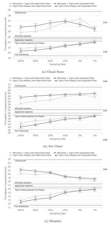
Figure 4: RQ1: Throughput by Sampling Rate. Performance of each application executed with and without APLCache using varying monitoring configuration.
