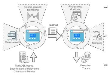
Figure 1: Overview of the Two-phase Monitoring Approach. It shows the input provided in the first phase (Coarse-grained Monitoring) and the resulting output of the second phase (Fine-grained Monitoring).
