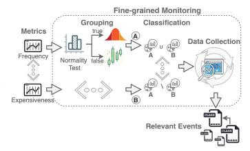
Figure 2: Fine-grained Monitoring Steps. Illustration of the three steps that comprise the fine-grained monitoring: Grouping, Classification and Data Collection.
