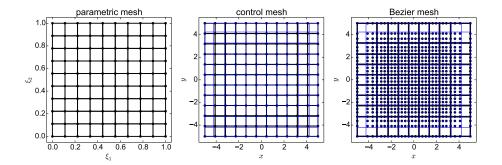
Figure 3: From left to right: parametric mesh (tensor product of knot vectors), control mesh, Bézier mesh. The corner vertices of Bézier mesh elements form the topological Bézier mesh. The thin blue lines are iso-lines of the NURBS parametrization.
