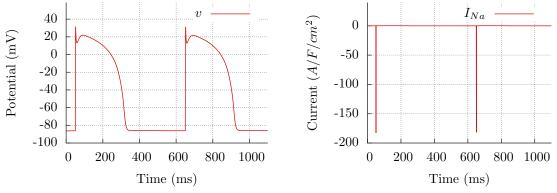
Figure 5: Two consecutive action potentials for the TNNP model: transmembrane potential v (left) and the fast sodium current  $I_{\text{Na}}$  (right), that is the main component of  $I_{\text{ion}}$  during the fast upstroke of the action potential.
