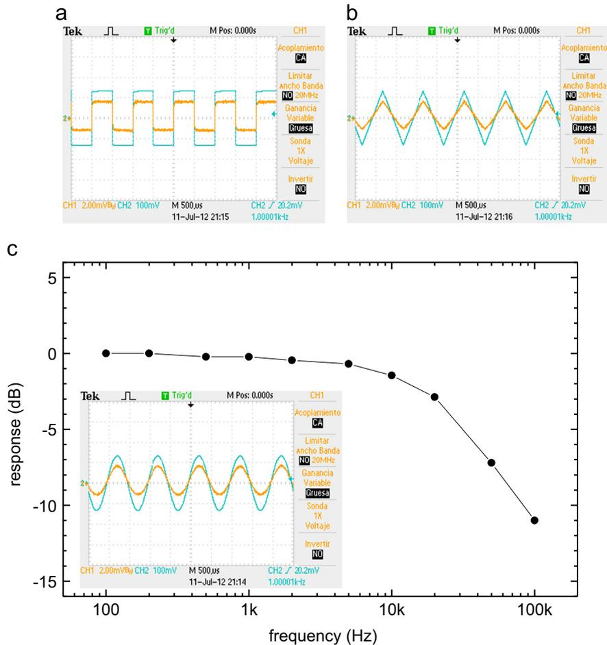
**Fig. 7.** AC behavior of the CNM 2.5  $\mu\text{m}$  based devices as current sensors: (a) output for a square wave (1 kHz) driven current, (b) output for a triangular wave (1 kHz) driven current, and (c) frequency response to a sinusoidal driven current and output for such a wave at 1 kHz.
