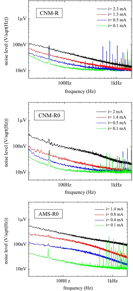
Fig. 4. Noise level (amplitude spectral density, ASD) at several bias currents for the different devices: CNM-R, spin valve onto current strip in a CNM chip; CNM-R0, spin valve onto free substrate in a CNM chip; AMS-R0, spin valve onto free substrate in an AMS chip.
