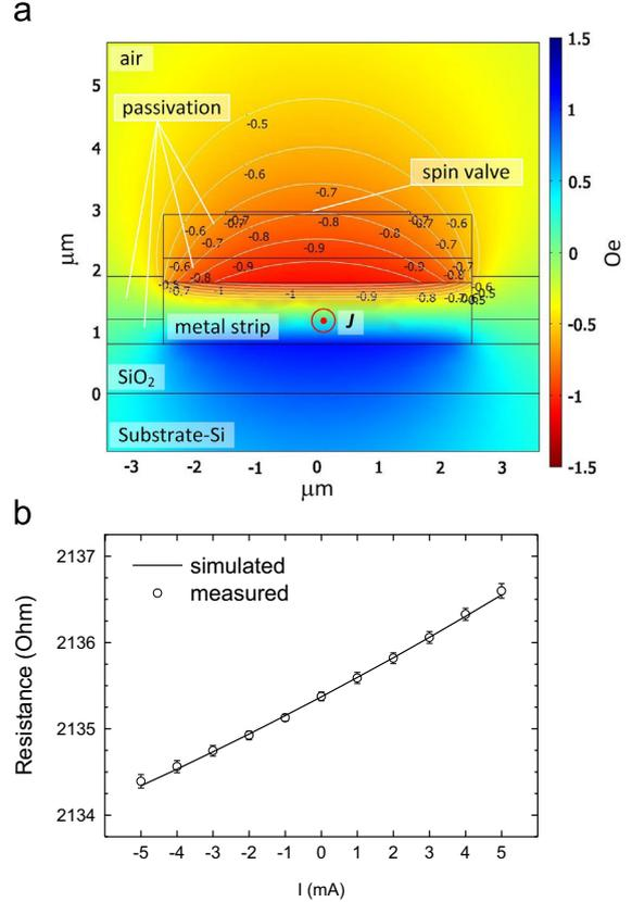
**Fig. 6.** 2D-FEM model of the CNM 2.5  $\mu\text{m}$  based devices as current sensors: (a) model description including magnetic field distribution, (b) resistance of the spin valve against the driven current: experimental data and simulation results.
