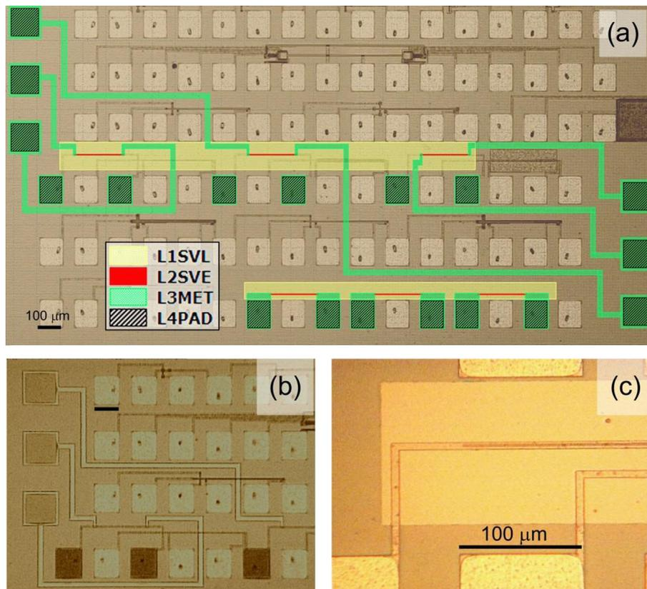
Fig. 2. Micrographs of the CNM chip with spin valves: (a) detailed masks, (b) general view of the finalized process, and (c) detail of a spin-valve onto a metallic strip.
