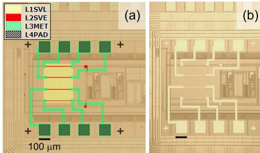
Fig. 1. Micrographs of the AMS chip with spin valves: (a) detailed masks, and (b) finalized process.
