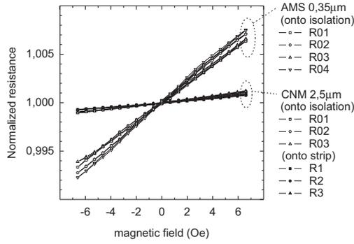
Fig. 3. Resistance of the deposited spin valve against the external magnetic field.
