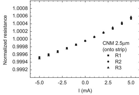
**Fig. 5.** Resistance of the deposited spin valve against the driven current in a CNM 2.5  $\mu\text{m}$  technology chip.
