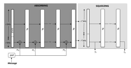
Figure 2: The sponge construction implemented by the hash function
