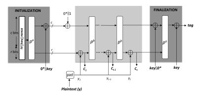
Figure 4: Encryption operation in ASCON
