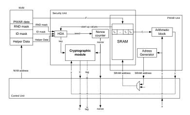
Figure 5: Architectural scheme of the proposed CMOS sensor
