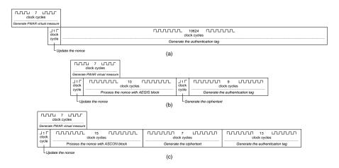
Figure 8: Timing of trusted virtual sensing mode for (a) HMAC, (b) AEGIS, (c) ASCON
