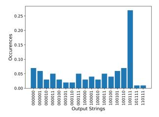
Figure 8: Top 20 outcomes from executions of the Bernstein-Vazirani program for the hidden bitstring "00111" (See Figure 6). The program qubits are measured in the order P5, P0, P1, P2, P3, P4 since P5 is expected to be 1. The required bitstring dominates the output distribution.
