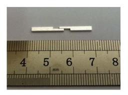
Fig. 1 Prepared sintered nano-silver lap-shear structure
