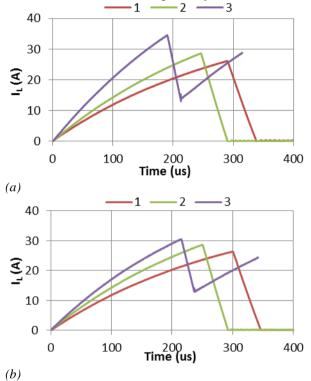
Fig. 4. Single pulse UIS waveforms at  $T_{CASE}$  (a) 90°C and (b) 150°C,  $V_{DD} = 400V$  with various L values and constant  $E_{AV}$
