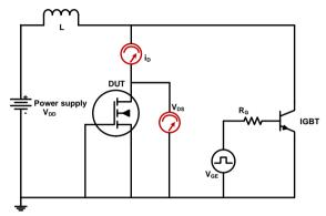
Fig. 1. UIS test circuit schematic
