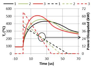
Fig. 7. Simulation of Junction temperature for test conditions from Table 3 at  $V_{DD} = 800V$ .
