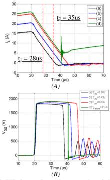
Fig. 8. UIS electrical waveforms: (A)  $I_L$  and (B)  $V_{DS}$ , with  $T_{CASE} = 27^{\circ}C$ ; L = 1.8mH; (a)  $V_{DD} = 140V$ ,  $t_{ON} =$ 200us (b)  $V_{DD}$ =180V,  $t_{ON}$ =200us (c)  $V_{DD}$ =200V, ton=220us; (d) V<sub>DD</sub>=200V, ton=230us.
