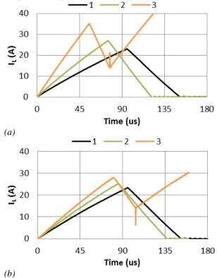
Fig. 5. Single pulse UIS waveforms at  $T_{CASE}$  (a) 90°C and (b) 150°C,  $V_{DD} = 800V$  with various L values and constant  $E_{AV}$
