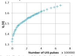
Fig. 11. Evolution of body diode forward voltage (V<sub>f</sub>) as a result of repetitve UIS stress
