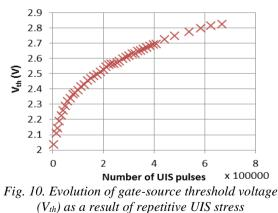
Fig. 10 shows that the  $V_{TH}$  has a positive shift as the number of UIS pulses increase. The shift of the  $V_{TH}$  is
