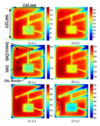
*Fig.* 9. Thermal maps taken during UIS tests of Fig. 8. The time instants are  $t_1=28us$ ,  $t_2=35us$ .
