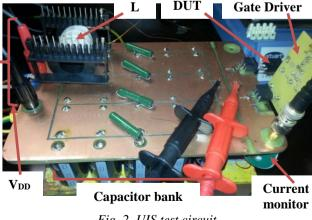
Fig. 2. UIS test circuit
