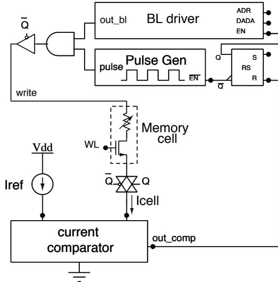
Fig. 4. Write assist circuit FMG/SET operation
