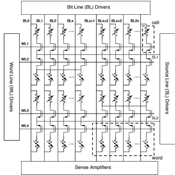
Fig. 3. Elementary memory array used for simulations
