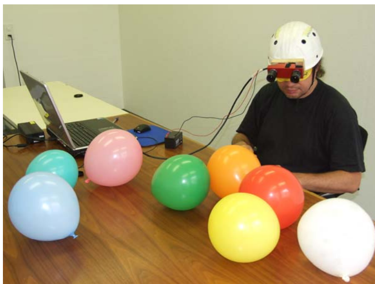
Figure 4. The See ColOr stereoscopic camera prototype.
