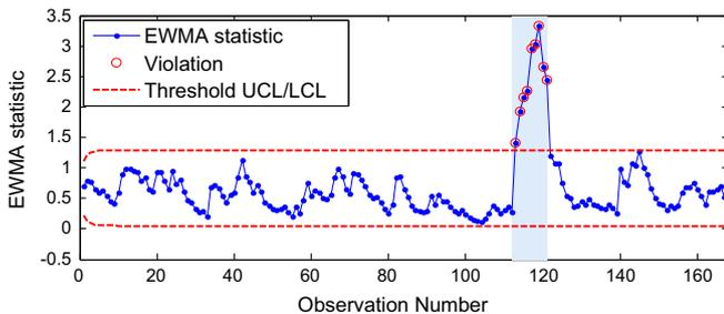
Fig. 12. Time evolution of the EWMA statistic in the presence of an abnormal situation (Case A<sub>1</sub>).
