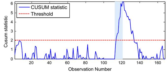
Fig. 14. Time evolution of the CUSUM statistic in the presence of an abnormal situation (Case A<sub>2</sub>).
