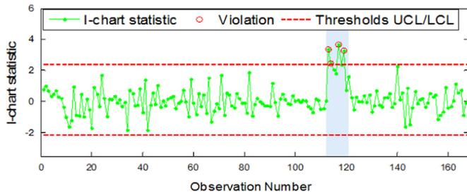
Fig. 10. Time evolution of the Shewhart I-chart statistic in the presence of an abnormal situation (Case A<sub>1</sub>).
