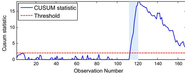
Fig. 11. Time evolution of the CUSUM statistic in the presence of an abnormal situation (Case A<sub>1</sub>).
