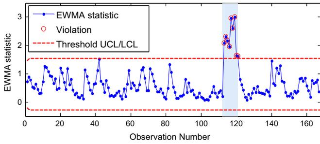
Fig. 15. Time evolution of the EWMA statistic in the presence of an abnormal situation (Case A<sub>2</sub>).
