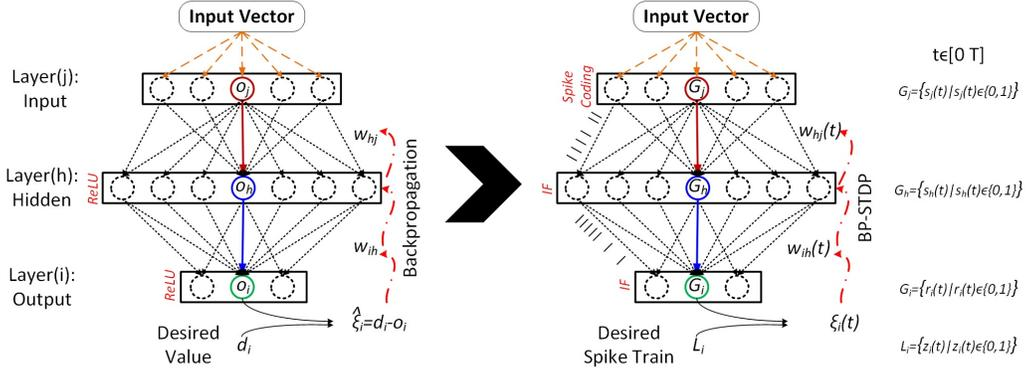
Figure 2: The 2-Layer, conventional (left) and spiking (right) network architectures. The SNN receives spike trains representing input feature values in  $T$  ms. The learning rules and the network status in the SNN are specified by an additional term as time ( $t$ ). The formulas and parameters are discussed in Eqs. 9 through 21.
