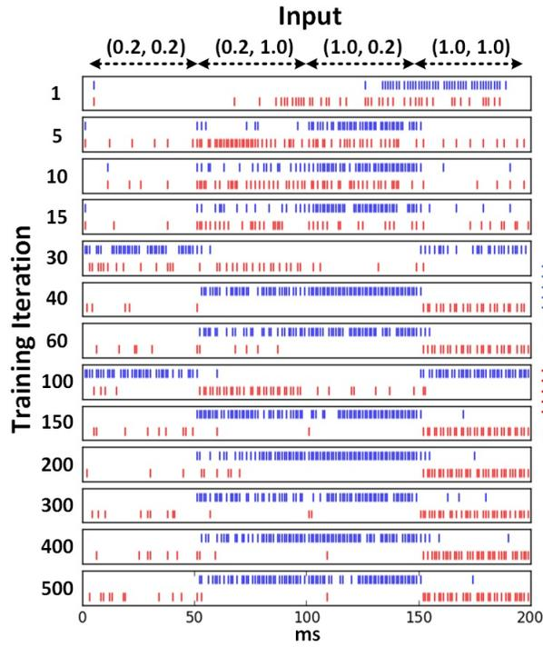
Figure 4: Spike trains released from the output neurons in response to four pairs of spike trains representing  $\{(0.2, 0.2), (0.2, 1), (1, 0.2), (1, 1)\}$  values in 1 through 500 iterations. We used high spike rates for better visualization.
