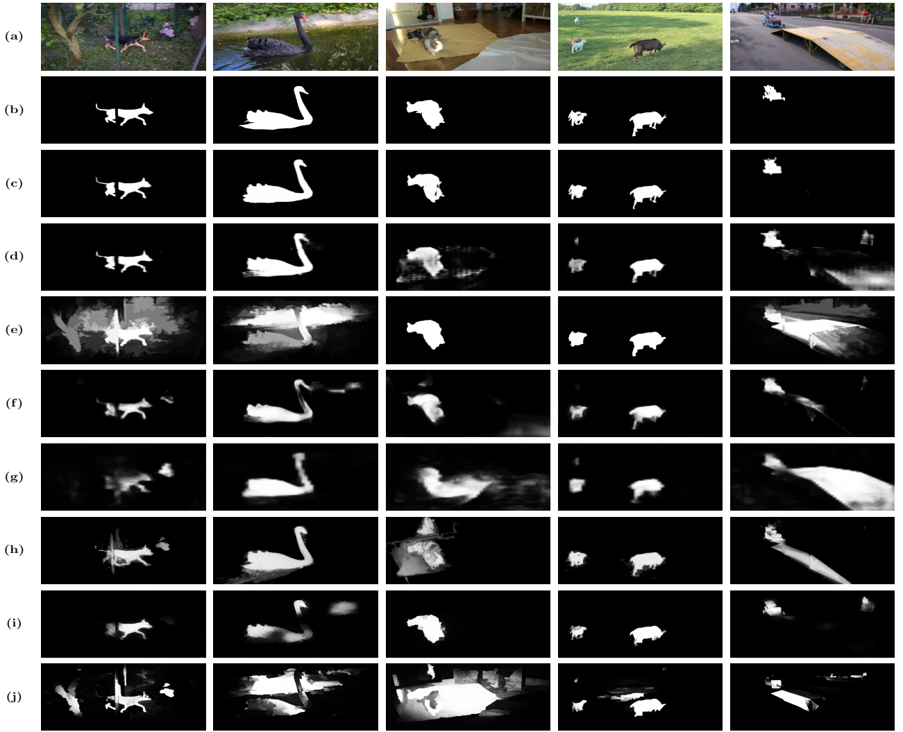
Figure 3: Visual comparison of dynamic saliency maps. Top-down: (a) Original images, (b) ground truth of salient objects, (c)-(j) detected outcomes by the proposed CFCN-MA, PDBM, MBNM, FGRN, DLVS, SCNN, SCOM, and MSTM, respectively.
