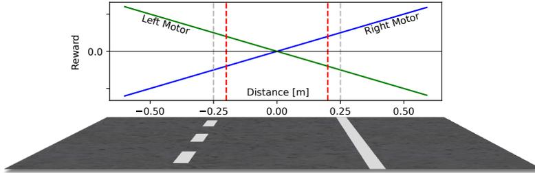
Figure 10: Reward given by the R-STDP controller: It is defined for each motor individually as a linear function of the lane center distance scaled by a constant  $c_r$ . The lane markings are  $0.25\text{ m}$  away from the lane center. If the robot goes further than  $0.2\text{ m}$  from the lane center, episodes are terminated and the robot is positioned at its starting position.
