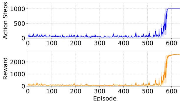
Figure 11: Scenario 1: After 500 episodes, the robot learns to follow the lane without triggering a reset. Episodes are limited to 1,000 action steps. The accumulated rewards collected in 1,000 action steps still improve after the robot has reached the step limit.
