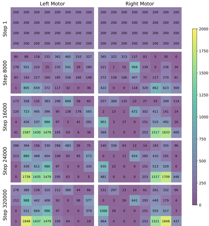
Figure 15: Scenario 1. Learning progress of the R-STDP controller over every 8,000 steps (1 step = 50 ms). Learned connection weights to the left and right motor neuron of the R-STDP controller are shown in last row after 30,000 simulation steps.
