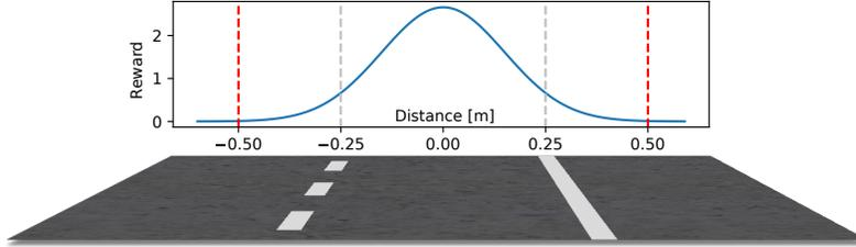
Figure 7: Reward given in the lane-keeping task. It is defined as a Gaussian distribution over the distance to the center of the lane with a standard deviation of  $\sigma = 0.15$  and mean at 0. The lane markings are  $0.25\text{ m}$  away from the lane center. If the robot goes further than  $0.5\text{ m}$  from the lane center, episodes are terminated and the robot is positioned at its starting position.
