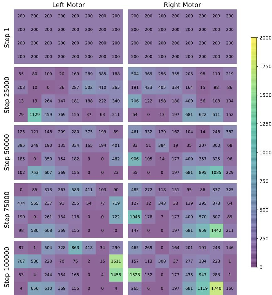
Figure 19: Scenario 3. Learning progress of the R-STDP controller over every 25,000 steps (1 *step* = 50 *ms*). Learned connection weights to the left and right motor neuron of the R-STDP controller are shown in last row after 100,000 simulation steps.
