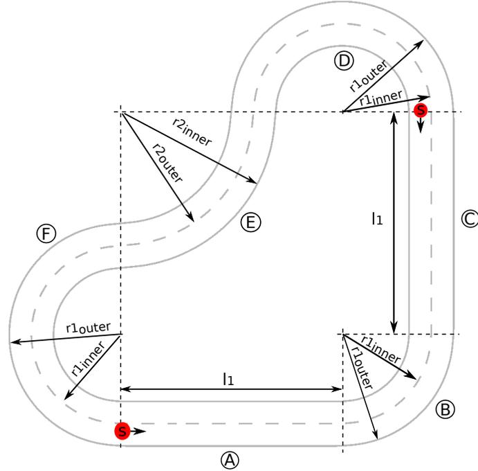
Figure 3: Scenario 1: The simple lane-keeping scenario consists of a road with two lanes (inner and outer) and six different sections A, B, C, D, E, and F. Starting positions are marked with  $S$ . Dimensions:  $r1_{inner} = 1.75\text{ m}$ ,  $r2_{inner} = 3.25\text{ m}$ ,  $r1_{outer} = 2.25\text{ m}$ ,  $r2_{outer} = 2.75\text{ m}$ ,  $l_1 = 5.0\text{ m}$ .
