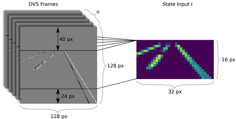
Figure 6: Conversion of consecutive DVS frames into state input for reinforcement learning. This is done by dividing the original  $128 \times 128$  DVS frames into small  $4 \times 4$  regions and counting every event over consecutive frames regardless of the polarity. Furthermore, the image is cropped at the top and bottom, resulting in a  $32 \times 16$  image.
