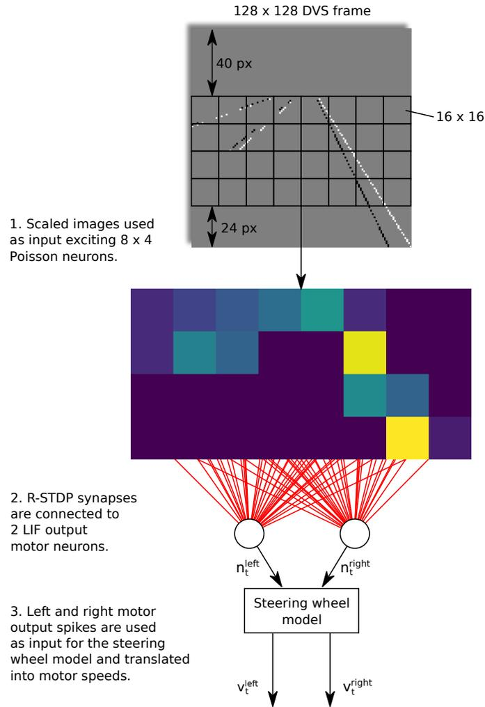
Figure 9: Network architecture of the R-STDP implementation using DVS frames as input.
