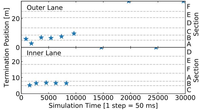
Figure 16: Scenario 1. Termination position of the robot at each trail is marked by a star. During the first 10,000 simulation steps, the robot triggers resets at each trial in the first turn in both directions. Afterwards, it has successfully learned how to follow the lane, only triggering a reset when a complete lap is finished.
