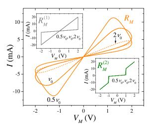
Figure 2: Current-voltage characteristics of device models considered in this Letter. Frequency-dependent pinched hysteresis loops of an actual memristive model (in the center) contrast with the frequency-independent loops of type 1 model (top left inset) and non-hysteretic characteristics of type 2 model (bottom right inset). This plot was obtained using the same model parameters as in Fig. 1;  $V_M(t)=2\sin(2\pi\nu_i t)$  V;  $\nu_0=1/T$ .
