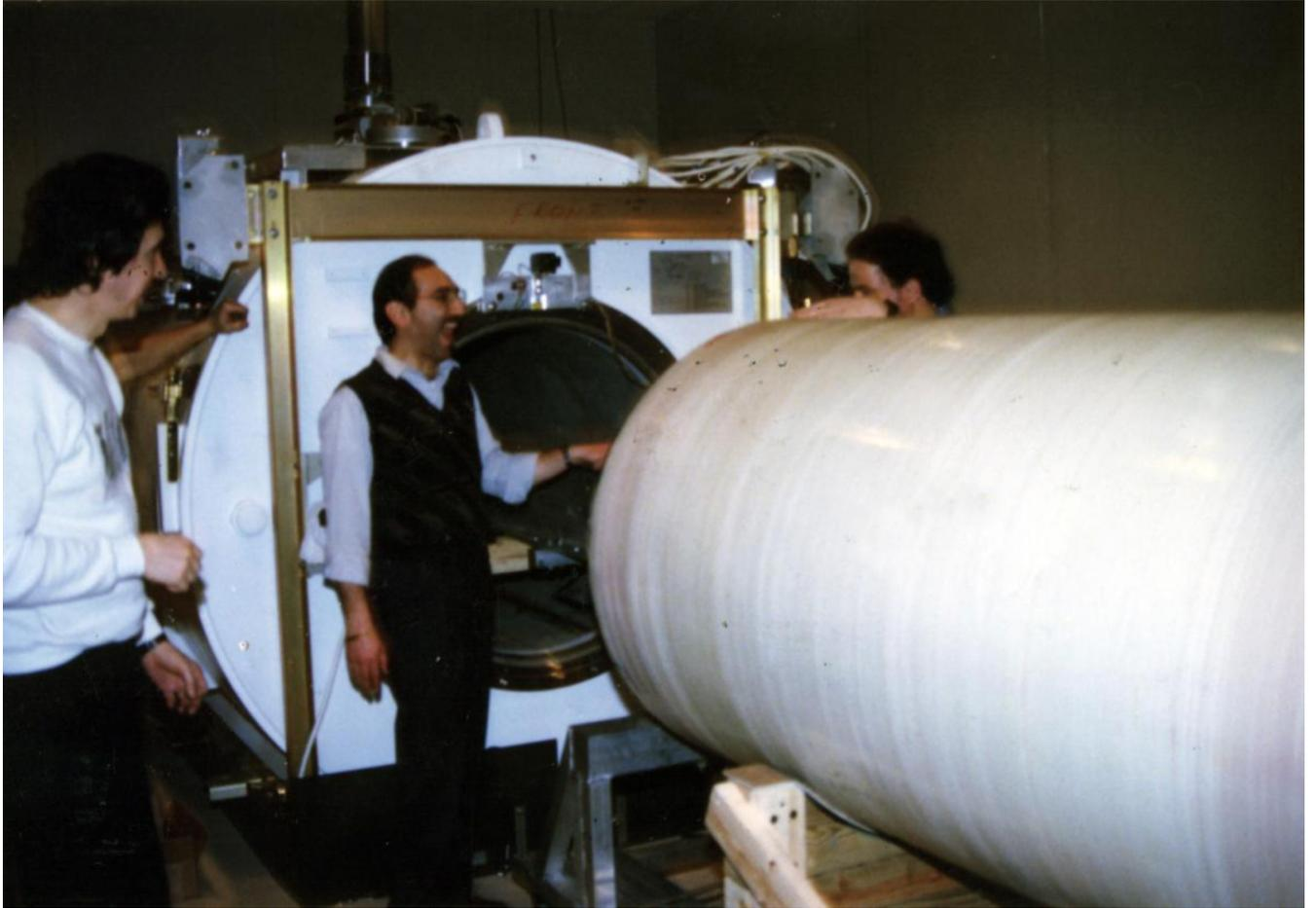
**Figure 1.** Richard Rzedzian (left), Robert Weisskoff (right) inserting the hand-wound, epoxy-covered, prototype echo planar gradient coil into the General Electric Signa scanner at Advanced NMR Systems in 1989.
