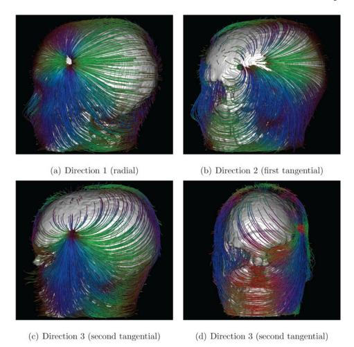
Figure 6. Streamlines depict the electrical flow field in the Skull-Hole-Model
