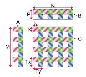
Figure 9: 2-D block-cyclic distribution for parallel matrix multiplication diagram. TX and TY are the dimensions of the 2-D thread grid.
