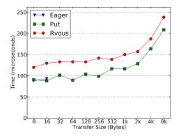
Figure 4: Comparison of Data Transfer Mechanisms (Broadcast performance on 2048 cores of the Cray XT4)
