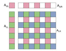
Figure 12: Cholesky Factorization Diagram with 2D blockcyclic distribution. The matrix is partitioned into 4 quadrants: a small upper left corner  $(A_{UL})$ , a tall skinny lower left corner  $(A_{LL})$ , a short and wide upper right corner  $(A_{UR})$ , and a large lower right corner  $(A_{LR})$ .
