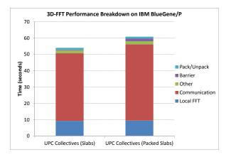
Figure 18: 3-D FFT (NAS FT) Performance Breakdown on IBM BlueGene/P
