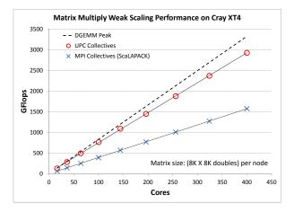
Figure 10: Matrix Multiply Performance on 400 cores of Cray $\rm XT4$
