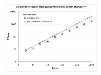
Figure 14: Cholesky Factorization Performance on 2048 cores of IBM BlueGene/P
