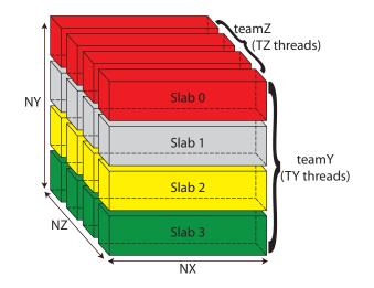
Figure 15: 2-D data partitioning for 3-D FFT. A thread owns  $\frac{NZ}{TZ}$  planes and  $\frac{NY}{TY}$  rows of NX points where the T threads are laid out in a  $TY \times TZ$  thread grid.
