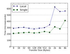
Figure 2: Comparison of Data Transfer Mechanisms (Broadcast performance on 2048 cores of the Cray XT4)
