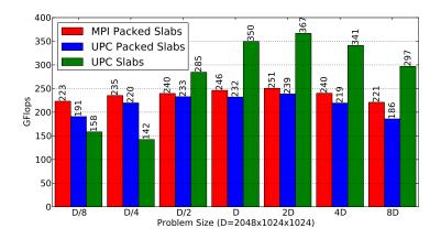
Figure 16: 3-D FFT Performance on 1024 cores of Cray XT4
