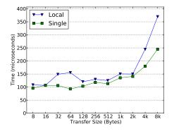
Figure 3: Comparison of Data Transfer Mechanisms (Broadcast performance on 1024 cores of the Sun Constellation)
