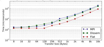
Figure 8: Comparison of Exchange Algorithms (2k cores of IBM BlueGeneP)
