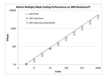
Figure 11: Matrix Multiply Performance on 2048 cores of IBM BlueGene/P
