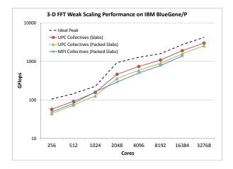
Figure 17: 3-D FFT (NAS FT) Performance on 32K-core IBM BlueGene/P. The UPC Slabs algorithm uses the UPC non-blocking exchange (alltoall) collective. The UPC Packed Slabs algorithm uses the UPC blocking exchange (alltoall) collective. The MPI Packed Slabs algorithm uses the MPI blocking alltoall collective.
