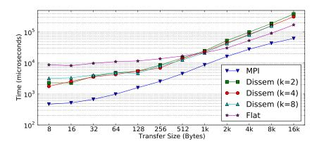
Figure 6: Comparison of Exchange Algorithms (512 cores of Cray XT4)
