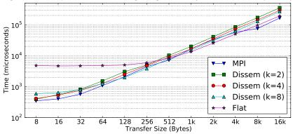
Figure 7: Comparison of Exchange Algorithms (256 cores of Sun Constellation)
