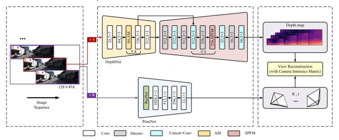
Fig. 2. The detailed network architecture of our SAM-Net. PoseNet outputs the 6-DoF relative poses. DepthNet outputs 4 scale depth maps. Except for the maximum scale depth map of the last layer, the depth maps of the other three scales are outputs from the last three SPFMs of the network.
