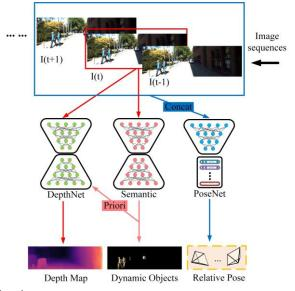
**Fig. 1.** Diagram of the proposed SAM-Net, which consists of the DepthNet and the PoseNet, taking respectively the current frame and the adjacent frames from a monocular image sequence as input for depth/pose estimation and object detection. After training the model in a totally self-supervised manner, we can estimate the pixelwise depth map, camera's ego-motion, and detect dynamic objects to generate the semantic probability map.
