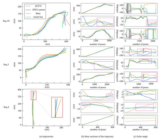
Fig. 8. Trajectories of KITTI sequences #03, #04 and #10 from our model (SAM-Net), SAM-Net without SPFM and AM (Base), SfM-learner [10] and ground-truth trajectories (KITTI) (a). As shown in (b) the three sections of the 3-D trajectory and (c) the Euler angle, our pose prediction is closer to the ground truth even when the SfM-learner failed [10] (purple rectangle). Moreover, after introducing the semantic prior information, pose estimation has achieved better results.
