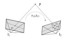
**Fig. 5.** An illustration of the differentiable image warping process of adjacent frames (pairwise matching and epipolar geometry). We use the differentiable bilinear sampling mechanism proposed by [37], which linearly interpolates the values of the 4-pixel neighbors of  $p_2$  to approximate the photometric of  $p_2$ .
