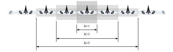
Fig. 3. Graphical representation of a linear cellular array with cooperating BS clusters.
