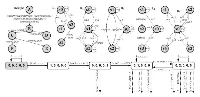
Figure 2: An example of a product recipe (top left), and simplified labelled transition systems  $R_1, \ldots, R_5$  modelling the resources in our assembly platform (top right). States  $s\theta$  and A are initial states. A fragment of the associated production topology is shown in the bottom figure.
