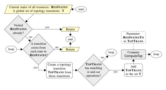
Figure 6: The flowchart for function ComputeTop. A dashed rectangle is a comment, a normal rectangle depicts a processing step, a coloured rectangle depicts the invocation of a function defined as a flowchart, a diamond depicts a decision point, a parallelogram depicts an input/output, and an ellipse depicts the start/end or a section of a flowchart.
