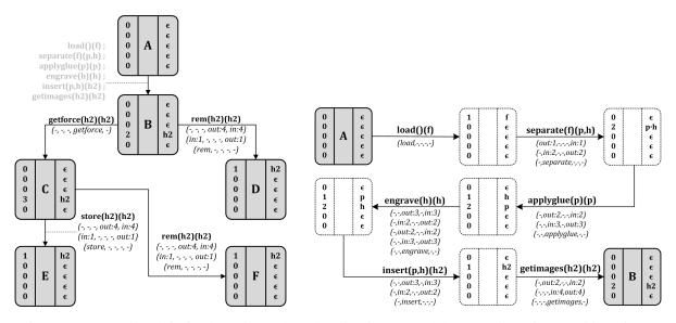
Figure 4: A controller (left) for the recipe and topology in Figure 2, and the controller's first transition (right).
