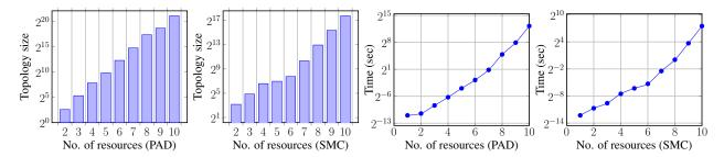
Figure 10: The size of the computed topology (log-scale) with an increasing number of resources for the PAD and SMC (the two graphs on the left), and average CPU time (log-scale) with an increasing number of resources for the PAD and SMC (the two graphs on the right).
