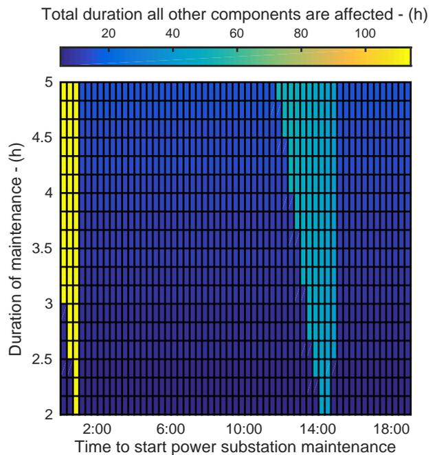
Figure 15: Plot showing the total duration that CISs components are affected with respect to the start time and the duration of a planned maintenance at the substation.
