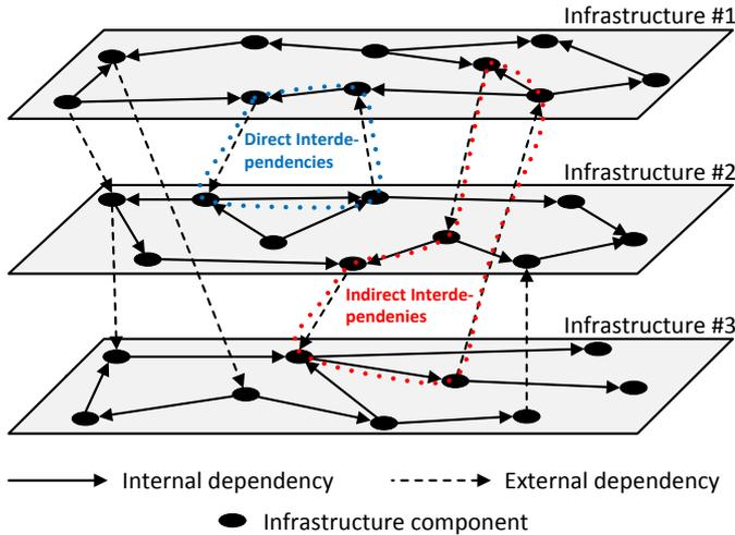
Figure 2: CISs consist by a large number of components which have internal and external dependencies among them, forming direct and indirect interdependencies between CISs.
