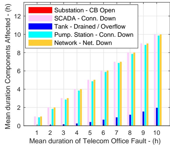
Figure 14: Plot showing how the duration of a telecom central office fault affects all the other CISs components.
