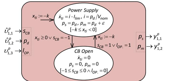
Figure 6: Open hybrid automaton for the power distribution substation.
