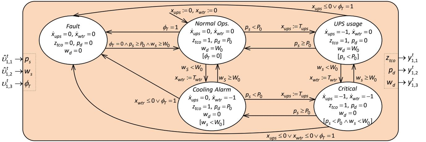
Figure A.18: Open hybrid automaton for the telecom central office.
