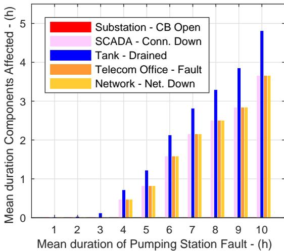
Figure 13: Plot showing how the duration of a water pumping station fault affects all the other CISs components.
