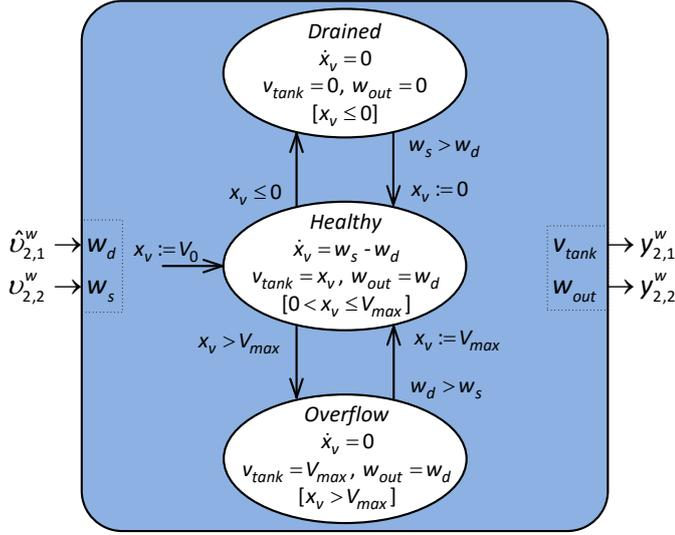
Figure A.16: Open hybrid automaton for the water tank.
