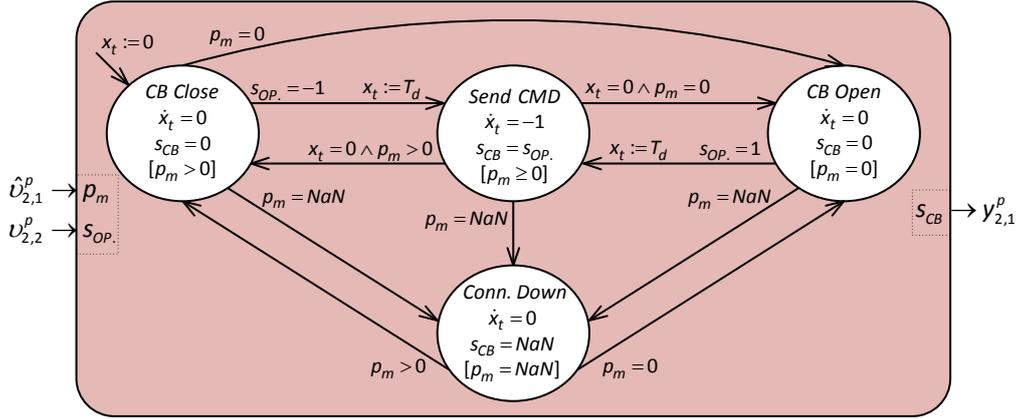
Figure 7: Open hybrid automaton for the power SCADA.
