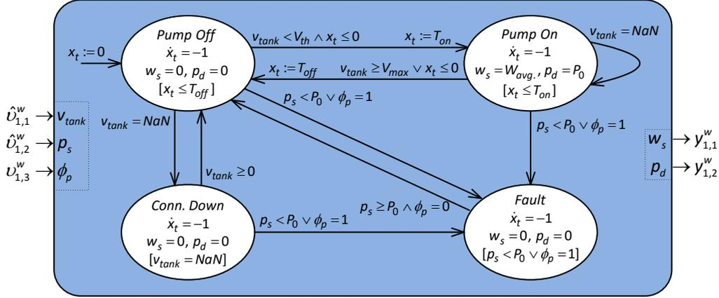
Figure A.17: Open hybrid automaton for the water pumping station.
