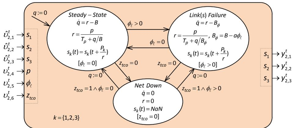
Figure B.19: Open hybrid automaton for the telecommunications network.
