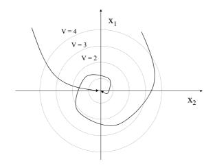
Figure 5: Trajectories Displaying First Order Asymptotic Stability.
