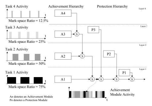
Figure 11: Standard Model for Behaviour Module Activity and Organisation within a Subsumption Architecture.
