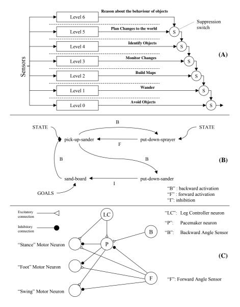
Figure 1: Behaviour-based System Architectures.
