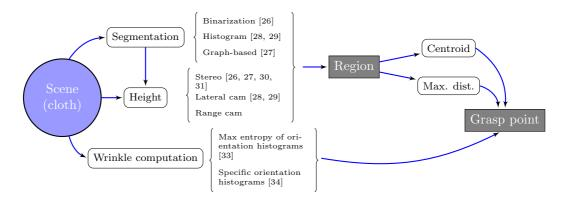
Figure 10: Different alternatives for generic GPL. Some references use only height (which justifies the arrow coming directly from the scene), whereas most works combine intensity image segmentation with height measure. The range camera is actually used in the wrinkle computation approaches, however it could constitute an alternative to stereo or lateral cameras for height computation.
