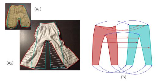
Figure 15: While in some cases a simple overlap ratio may suffice for assessing contour coincidence  $(a_1)$ , in others a great discrepancy may exist  $(a_2)$ . In such cases, the DTW algorithm provides a reasonable contour correspondence measure [23]. (b) Vertex-vertex (in blue) and vertex-edge correspondences between the two polygonal contours corresponding to the model and to the test image (adapted from [5] to the pants example).
