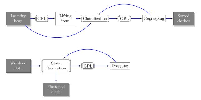
Figure 5: Basic laundry sorting and cloth flattening (by dragging) manipulation tasks, involving the surveyed perceptual actions. In the first, classification may eventually be made without lifting the object, by direct visual inspection. As for the flattening application, the type of cloth is assumed to be already known. Dragging is assumed to include the actual grasping and releasing actions.
