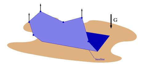
Figure 12: The points to be grasped are determined by the criterion of avoiding the deformation of the part of the cloth which is lifted, hanging vertically from the grippers: all the convex corners not on the baseline (i.e., not touching the ground) at which the negative gravity vector does not point inside the cloth polygon have to be grasped. These points are marked with an upward arrow in the figure.
