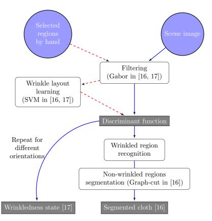
Figure 7: Cloth detection in a scene without prior knowledge. Monocular views are processed in both references.
