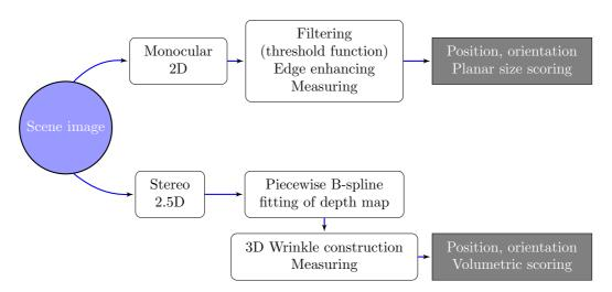
Figure 8: Different approaches for wrinkle measuring. On top, the purely planar procedure of [18], below the volumetric approach of [19].
