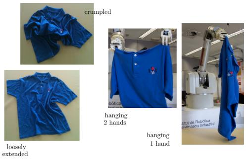
Figure 13: Different appearances of a garment in which classification and/or state recognition algorithms have been tested. Hanging states may, in turn, be just an arbitrary configuration of the garment held at any point, or belong to a finite set of discrete configurations corresponding to predefined grasp points.
