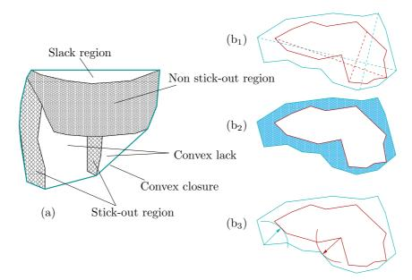
Figure 14: (a) Geometric features whose measurements and their ratios are used in [24]. (b) Some of the geometric features used in [27]: (b<sub>1</sub>) Eccentricity difference, where the eccentricity is measured in terms of the ratio between the maximum chord of the shape and the maximum chord which is perpendicular to the first; (b<sub>2</sub>) Difference in area (shaded region); (b<sub>3</sub>) Hausdorff distance between contours.
