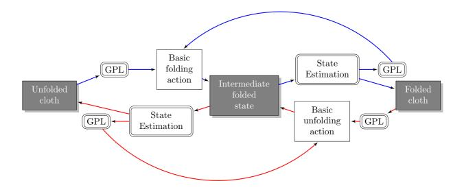
Figure 4: Basic folding and unfolding manipulation tasks, involving the surveyed perceptual actions. The extreme states are assumed to be known beforehand. Furthermore, the type of garment is also assumed to be known (otherwise, a Classification node should be placed before the first folding (or unfolding) action).
