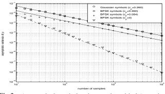
Fig.1 Asymptotic theoretical variance  $c_{\rho}$  given by (3) as a function of the circularity coefficient  $\rho$  for BPSK and Gaussian symbols  $s_t$  for P = 2 and 500 realizations of a Rayleigh channel whose three coefficients have same variance.
