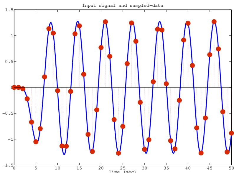
FIGURE 8. The original analog signal and its sampled-data
