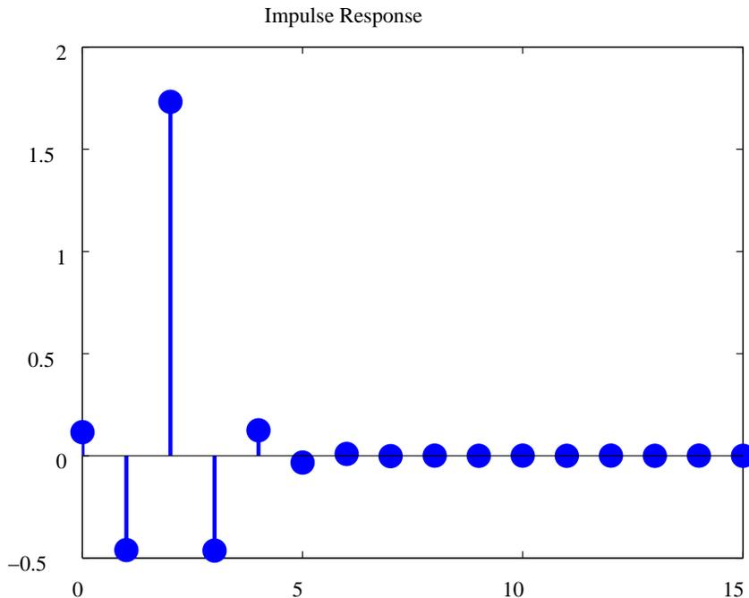
FIGURE 5. Impulse response of  $H^\infty$  optimal IIR filter  $\psi(z)$ **Table 2.**  $H^\infty$  norm of  $E(z)$
