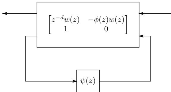
FIGURE 3. Block diagram for  $H^\infty$  optimization
