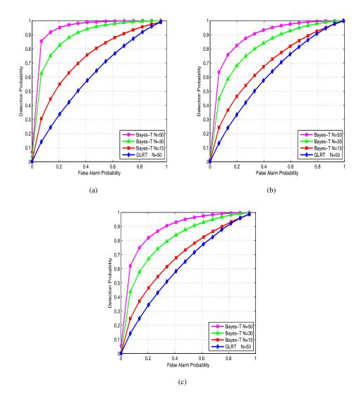
Figure 7: ROC curves for the Bayesian and GLRT detector with L=5, P=5 and different number of snapshots per sensing frame. (a) Stationary channel with SNR = -8 dB and  $\lambda=1.0$ . (b) Slowly time-varying channel with SNR = -8 dB,  $\lambda=0.97$  and  $\lambda_{ch}=0.90$ . (c) Fast time-varying channel with SNR = -8 dB,  $\lambda=0.97$  and  $\lambda_{ch}=0.10$ .
