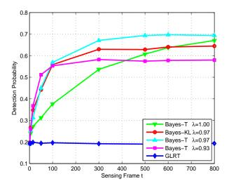
Figure 6:  $P_D$  for the Bayesian detector (Bayes-KL and Bayes-T) and the GLRT vs. the number of sensing frames in a fast time-varying channel. L = 5, P = 5, N = 50, SNR = -8 dB,  $P_{FA} = 0.1$ , and  $\lambda_{ch} = 0.1$ .
