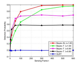
Figure 4:  $P_D$  for the Bayesian detector (Bayes-KL and Bayes-T) and the GLRT vs. the number of sensing frames in a time-invariant channel, L = 5, P = 5, N = 50, SNR = -8 dB and  $P_{FA} = 0.1$ .
