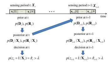
Figure 2: A Bayesian framework for spectrum sensing: the posteriors obtained after processing a sensing frame are employed as priors for the next sensing frame.
