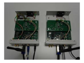
Figure 10: N210 Ettus devices with the XCVR2450 daugtherboard installed. A two-antenna cognitive receiver is composed of two N210 boards connected through a MIMO cable.
