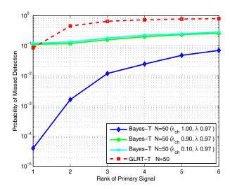
Figure 9: Probability of missed detection versus the rank of the primary signal P for both detectors with L=6 antennas, N=50, SNR = -8 dB and  $P_{FA}=0.1$ . A static time-invariant channel with  $\lambda=1.0$  using a KL posterior approximation, a slowly time-varying channel with  $\lambda=0.97$  and  $\lambda_{ch}=0.90$ , and a fast time-varying channel with  $\lambda=0.97$  and  $\lambda_{ch}=0.10$ .
