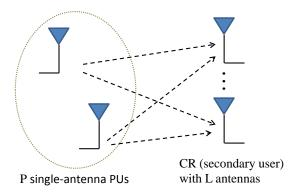
Figure 1: CR detection model: a cognitive user with L antennas tries to detect the presence of  $P \ge 1$  single-antenna PUs or, equivalently, a single P-antenna PU.
