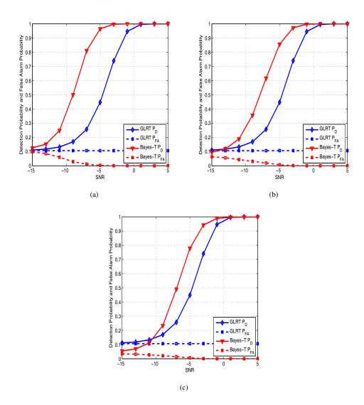
Figure 8:  $P_D$  and  $P_{FA}$  vs SNR with L=5 antennas, and N=50. (a) In a time-invariant channel ( $\lambda=1$  and  $\lambda_{ch}=1$ ). (b) In a slowly time-varying channel, ( $\lambda=0.97$  and  $\lambda_{ch}=0.95$ . (c) In a fast time-varying channel ( $\lambda=0.95$  and  $\lambda_{ch}=0.10$ ).
