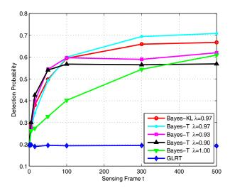
Figure 5:  $P_D$  for the Bayesian detector (Bayes-KL and Bayes-T) and the GLRT vs. the number of sensing frames in a slowly time-invariant channel. L = 5, P = 5, N = 50, SNR = -8 dB,  $P_{FA} = 0.1$  and  $\lambda_{ch} = 0.9$ .
