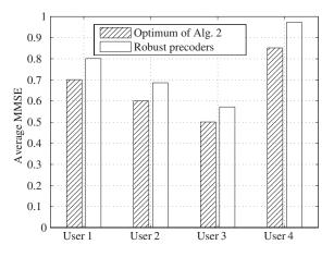
Fig. 7. Robust Transceiver: Average MMSEs for proposed Alg. 2 vs. Average MMSEs for Robust Transceivers.
