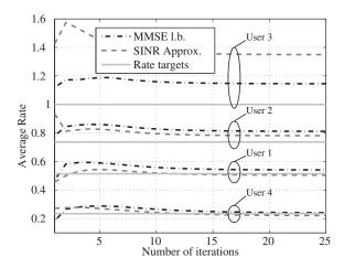
Fig. 4. Power Minimization: Rates vs. Number of Iterations.
