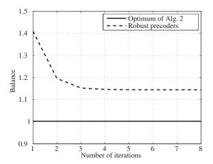
Fig. 6. Robust Transceiver: Balancing Level vs. Number of Iterations.
