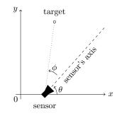
Fig. 7. Schematics of notations used to formulate control action space and detection probability in scenario 3 with spinning control actions.
