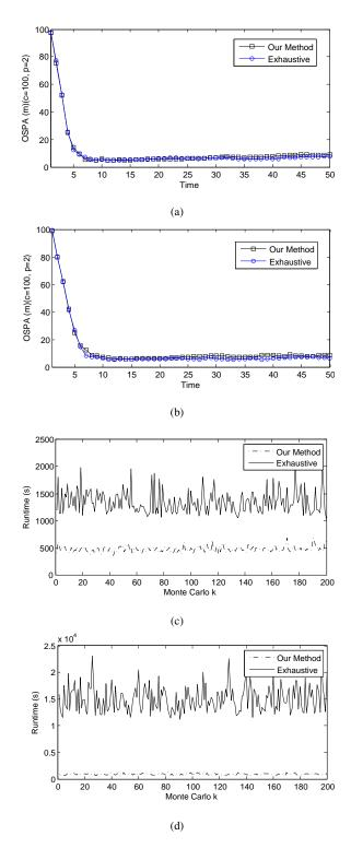
Fig. 3. (a) Average OSPA errors in scenario 1 for three sensors and (b) four sensors. (c) Run times for each time-step (averaged over 200 Monte Carlo runs) for three sensors and (d) four sensors.
