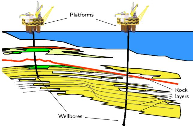
Figure 2: Platforms, wellbores, and rock layers; an illustration of the complex nature of petroleum reservoirs.
