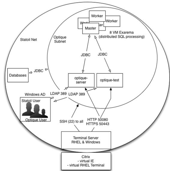
Figure 21: Optique platform server architecture at Statoil
