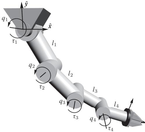
**Figure 5.2** A 4 degree-of-freedom serial chain robot parameterized using four generalized coordinates.
