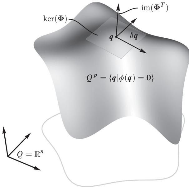
**Figure 5.5** The configuration space constrained-motion manifold,  $Q^p$ . All constraint-consistent virtual variations,  $\delta q$ , lie in the tangent space of  $Q^p$  and are orthogonal to the constraint forces.
