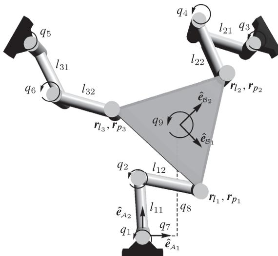
**Figure 5.8** Parallel mechanism consisting of serial chains with loop closures. The three elbow joints are actuated, while the remaining joints are passive.
