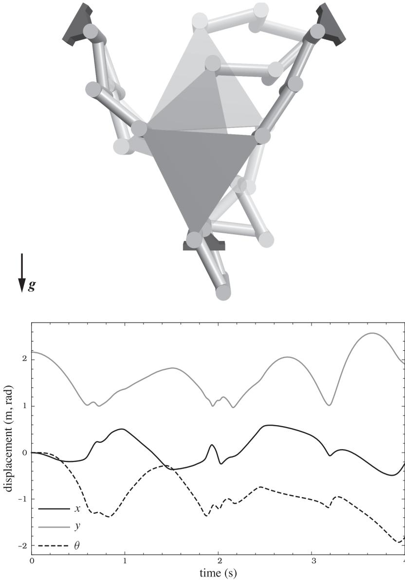
**Figure 5.9** (Top) Animation frames from the simulation of the parallel mechanism falling under gravity. (Bottom) Time history of the motion of the platform  $(x, y, \theta)$ .
