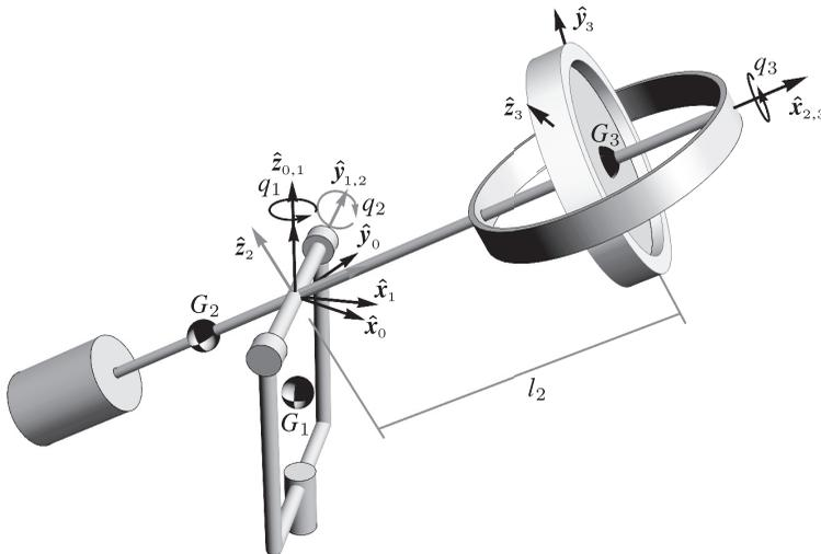
**Figure 5.11** A gyroscope supported by a two-axis gimbaled frame. The generalized coordinates,  $q_1$  and  $q_2$ , parameterize the gimbal frame, and  $q_3$  is the rotor angle. The rotor diameter is  $r$ .
