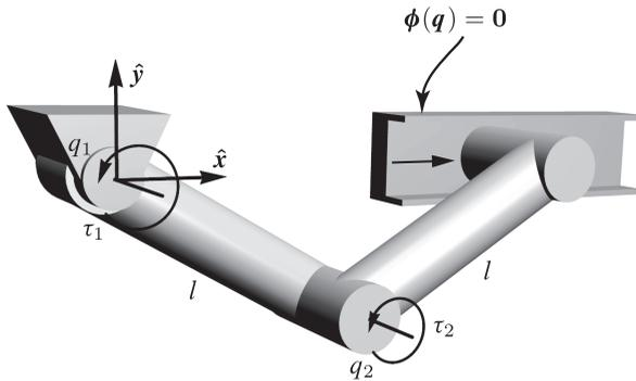
**Figure 5.15** A two-link planar slider-crank mechanism (Exercises 2, 6, and 8). The unconstrained system is parameterized by the generalized coordinates,  $q_1$  and  $q_2$ , with generalized forces,  $\tau_1$  and  $\tau_2$ . The link lengths are each  $l$  and the link masses are each  $M$ . The centers of mass are at the geometric centers of the links. The link rotational inertias are taken to be *zero*. Link 2 is constrained from translating in the  $\hat{y}$  direction.
