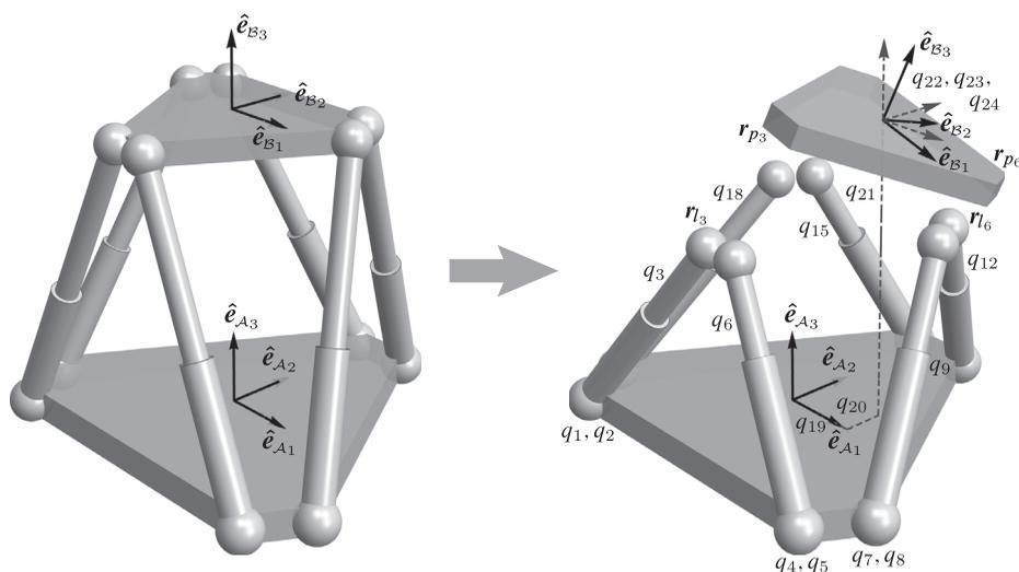
**Figure 5.6** (Left) Stewart platform actuated by six prismatic struts (remaining joints are passive). (Right) The closed-loop mechanism is cut at various locations to create serial chains described by the set of generalized coordinates,  $q_1, \dots, q_{24}$ .
