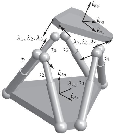
**Figure 5.7** Constraint forces associated with loop closures. Lagrange multipliers,  $\lambda$ , represent constraint forces at various locations between the serial chains to enforce the constraints associated with the loop closures.
