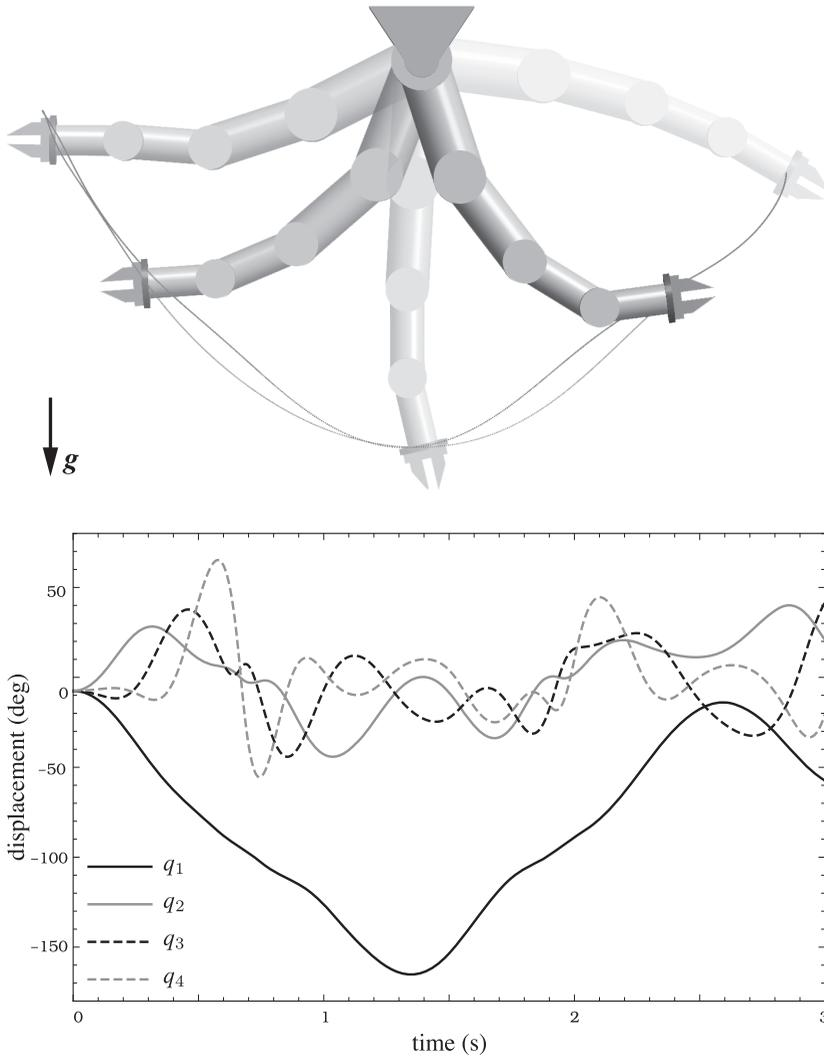
**Figure 5.3** (Top) Animation frames from the simulation of a serial chain robot. (Bottom) Time history of the robot generalized coordinates  $(q_1, q_2, q_3, q_4)$ .
