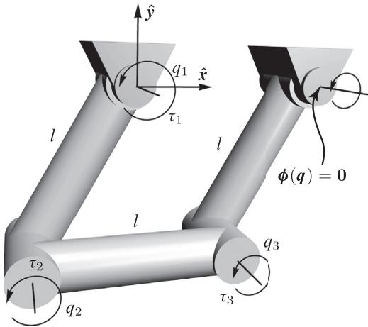
**Figure 5.16** A planar four-bar linkage (Exercise 3). The unconstrained system is parameterized by the generalized coordinates,  $q_1$ ,  $q_2$ , and  $q_3$ , with generalized forces,  $\tau_1$ ,  $\tau_2$ , and  $\tau_3$ . The link lengths are each  $l$  and the link masses are each  $M$ . The centers of mass are at the geometric centers of the links. The link rotational inertias are taken to be *zero*. The link 3 endpoint is constrained from translating.
