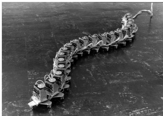
Fig. 1. The Active Cord Mechanism model ACM III.<sup>3</sup> By permission of Oxford University Press.
