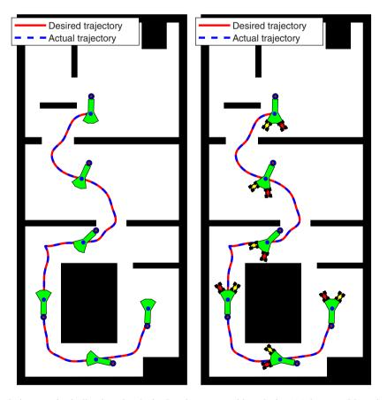
Fig. 12. Simulation results indicating the desired trajectory tracking during (a) human (blue circle with red center) moving the object (green) alone and (b) the proposed cooperative scheme (red and yellow robots). In both cases, the tracking is satisfactory (i.e., (a) RMS( $||e_p||_2$ ) = 0.0085 m, RMS( $\theta$ ) = 0.011 rad, (b) RMS( $||e_p||_2$ ) = 0.0089 m, RMS( $\theta$ ) = 0.012 rad, where  $\theta$  is the orientation.)
