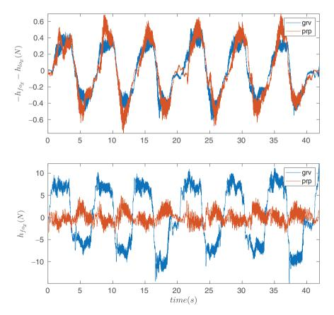
Fig. 5. Force owned to the object's motion and interaction force in x direction for gravity compensation (grv) and the proposed approach (prp).
