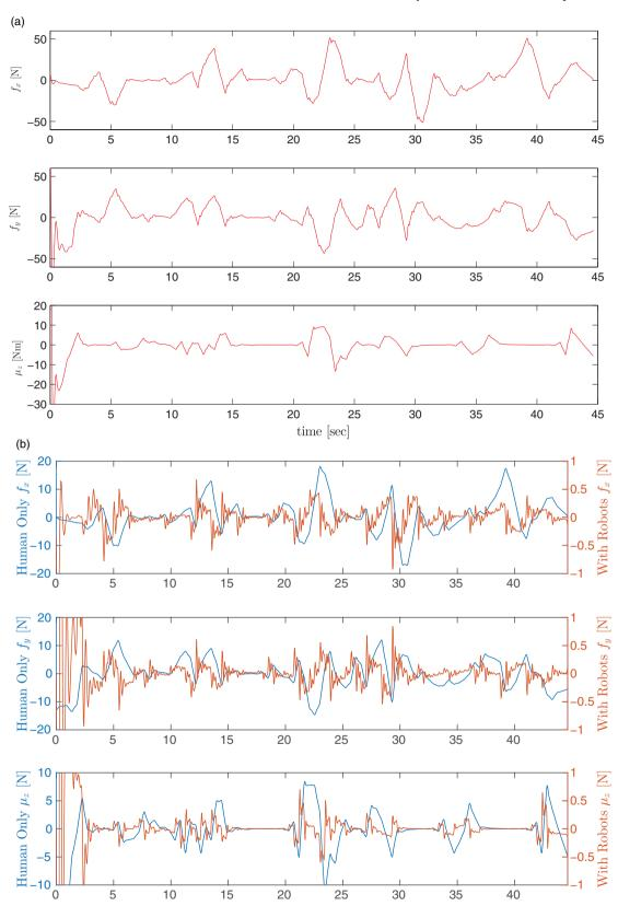
Fig. 13. Simulation results depicting (a) forces/torque exerted on the object's center by the robots, (b) the human effort both when human operates alone and when cooperates with the robots.
