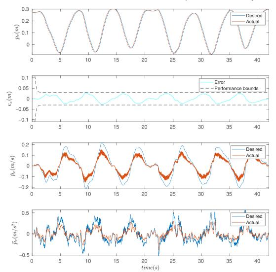
Fig. 4. Example of estimation in position, velocity and acceleration where *desired* is referring to the estimated signal and *actual* to the measured one.
