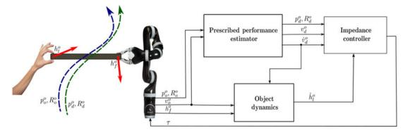
Fig. 2. Control diagram of the proposed method.
