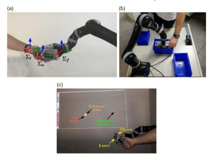
Fig. 3. (a) Cooperative transportation setup, (b) example of a task as described in the experiment of Section 4.1, the subject had to place the object inside every blue box starting from an arbitrary position, (c) the setup used for the experiments described in Section 4.2.
