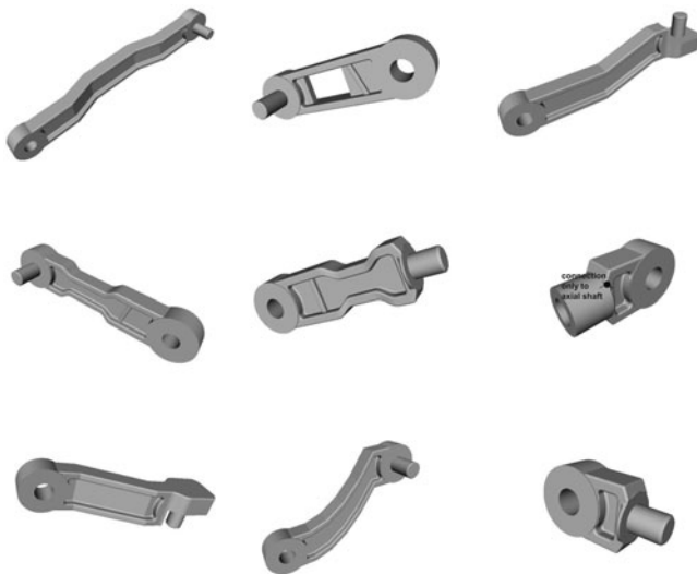
Fig. 20. Several solutions for robot arm links.
