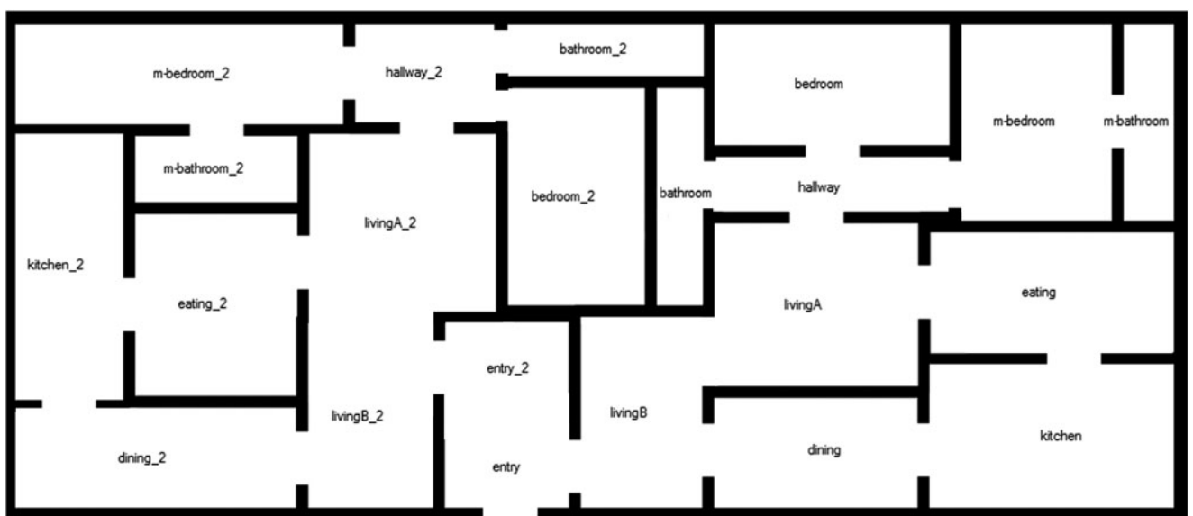
Fig. 12. Screenshot of a solution for two layout scenarios 3 (22 rooms) coupled via their entry rooms generated by the dense packing layout solver.
