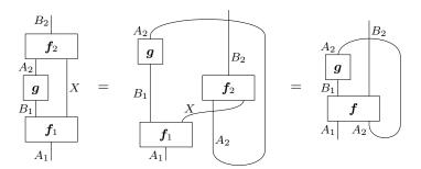
See e.g. [22] for more details. As it is possible to freely pass between f and  $f_1, f_2$ , one could equivalently define a comb as an equivalence class of pairs  $(f_1, f_2)$  which compose to give f, much like those considered in the construction of completely positive maps in [8].
