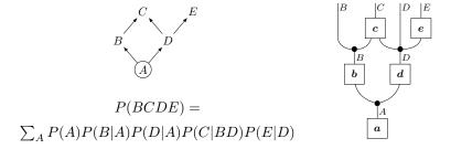
In general, a Bayesian network (with possible latent variables), is a string diagram in Stoch that (1) only has outputs and (2) consists only of copy maps and boxes which each have exactly one output.
