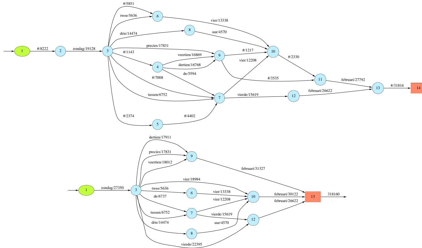
Figure 19: Word-graph and normalized word-graph for the utterance Zondag vier februari (Sunday Februari fourth). The special label # in the first graph indicates a pause transition. These transitions are eliminated in the second graph.
